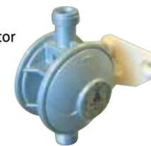
This caravan regulator is a two-stage regulator which can work with both Butane and Propane gas. It has built-in over-pressure protection and switching between different gas cylinders is achieved simply by changing the high pressure hose or adding a Gaslow adaptor on to the W20 inlet. It is manufactured to European standard 12867 which is now required for caravans and motorhomes built to EN1949.
