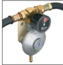
Designed for twin cylinder Propane systems conforming to the original British Standard, it is a manual changeover regulator complete with an integral mounting bracket. Comes standard with a hose nozzle but optional 5/16" and 3/8" compression fittings are available.
