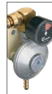
Regulator and bracket to be mounted with a single high-pressure 0.45metre hose which connects to the cylinder. For marine use, the regulator must be connected directly to the copper piping using either the 3/8" or 5/16" compression fitting.
