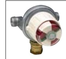
Simply screw this changeover on to your 30mbar regulator and it works with both Butane and Propane. When gas levels run low, the sensing device automatically changes to the reserve cylinder without interrupting the gas flow. The non-return valve allows disconnection of the empty cylinder without disrupting the supply.
