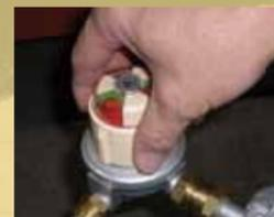
To change the empty cylinder, rotate the plastic indicator to the cylinder in use.
