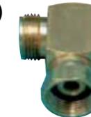
Designed to bring the W20 connection on 30mbar regulators round 90 degrees to help installation of Gaslow upgrade systems and/or high pressure hose connections in confined spaces.
